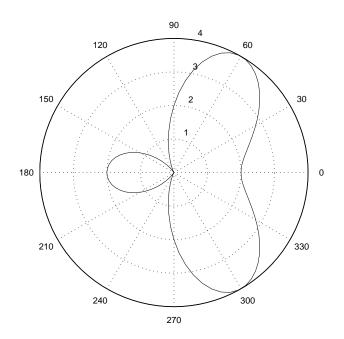
Next let's look at an example of pattern synthesis. In this example we want to use two antennas to produce no radiation in the north/south directions and maximum radiation in the east/west direction.
