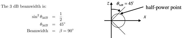
The direction of maximum radiation occurs at  $\theta = 90^{\circ}$  or perpendicular to the dipole.
