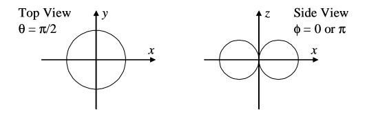
The power density of the Hertzian dipole decays with distance  $1/R^2$ .
