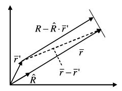
We can now do the integration for a half-wavelength dipole. A reasonable approximation for the current on a dipole is a sinusoid that goes to zero at the ends of the dipole wires, or  $\overline{J}(\overline{r}') = \hat{z}I_o\delta(x')\delta(y')\cos(kz'), -\lambda/4 \leq z' \leq \lambda/4$ . Then
