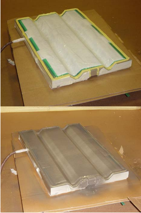
Figure 3 Parts with reasonably deep draws showing a conventional vacuum bag assembly and the bare tool
