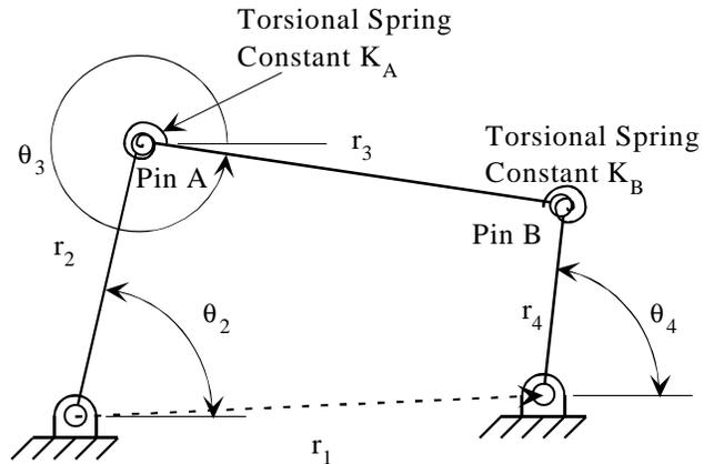
**Figure 9: A model of the four-link mechanism class chosen for the bistable micro-mechanism.**
