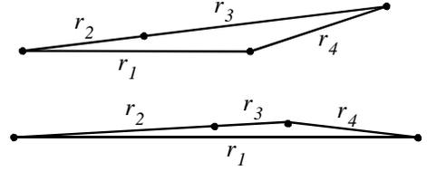
**Figure 4: A graphical representation near the limits required for  $\theta_2$  to be equal to  $\theta_3$ .**
