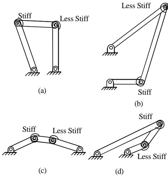
**Figure 10: Four possible mechanism configurations for bistable micro-mechanisms. (a) is Grashof, and (b), (c), and (d) are non-Grashof.**
