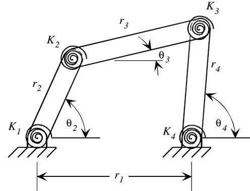
**Figure 2: A four-link mechanism with a torsional spring at each joint.**
