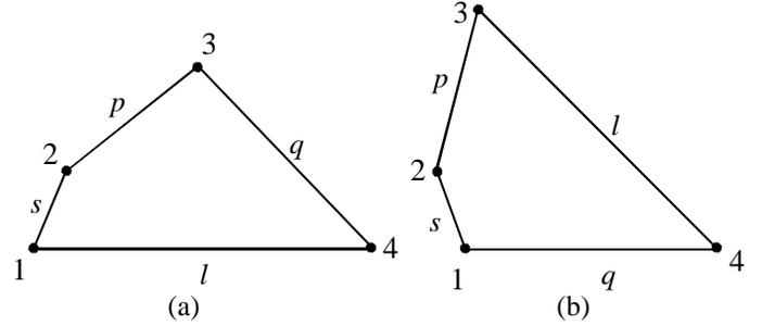
**Figure 5: The two kinematic chains which form a four-link mechanism.**
