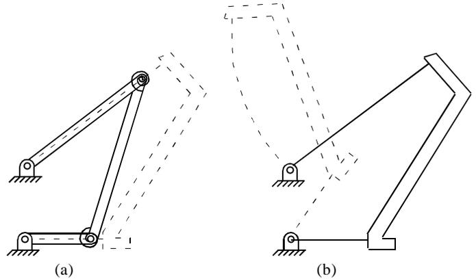
**Figure 11: An example of a bistable compliant micro-mechanism whose pseudo-rigid-body model is a non-Grashof four-link mechanism. (a) shows the mechanism and its pseudo-rigid-body model, and (b) shows the two stable positions.**
