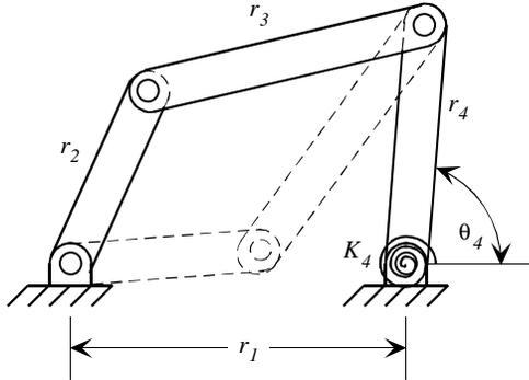
**Figure 3: The two different positions of a four-link mechanism for a given angle  $\theta_4$ .**
