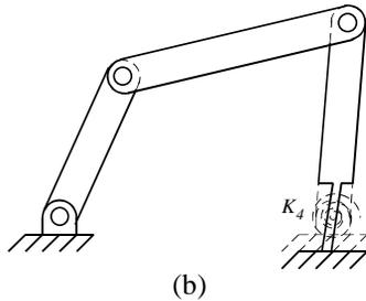
**Figure 6: A bistable four-link mechanism showing the two stable positions and one unstable position (a), and a compliant equivalent (b).**
