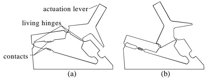
**Figure 8: Layout for a fully-compliant bistable switch as-fabricated (a) and closed (b). (Patent pending.)**
