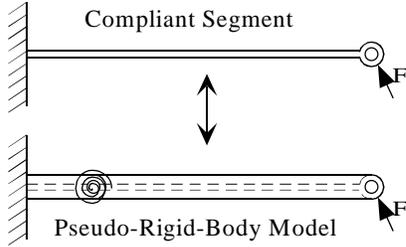
**Figure 1: The concept of the pseudo-rigid-body model. Compliant segments are modeled as rigid segments joined by pin joints, with torsional springs at the joints.**
