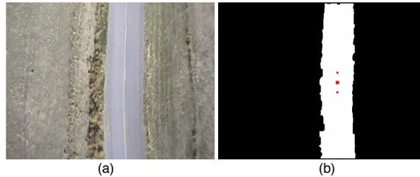
Figure 16: This figure shows one camera frame captured during the road following demonstration and the corresponding result of the classification algorithm.
