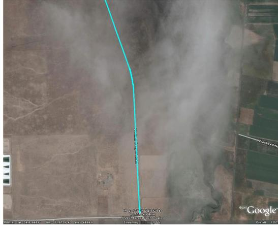
Figure 15: This figure is a map of Goshen Canyon Road in Mona, UT. The curvature of the road has a maximum amplitude  $\alpha = 400$  m so that the roll-angle constraint cannot be set below 5 degrees in order to follow the road at 70 m AGL.
