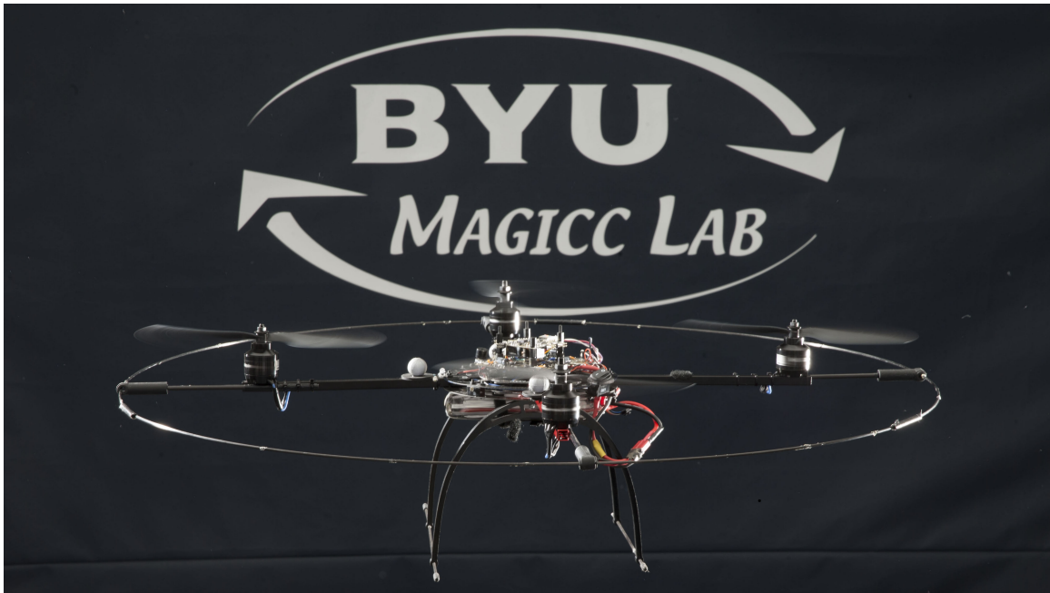
Figure 2. Hovering Quadrotor. A quadrotor from MikroKopter that was used in the experiments. The vehicle is hovering using the measurements from the motion capture system. ©Jaren Wilkey, BYU Photo
