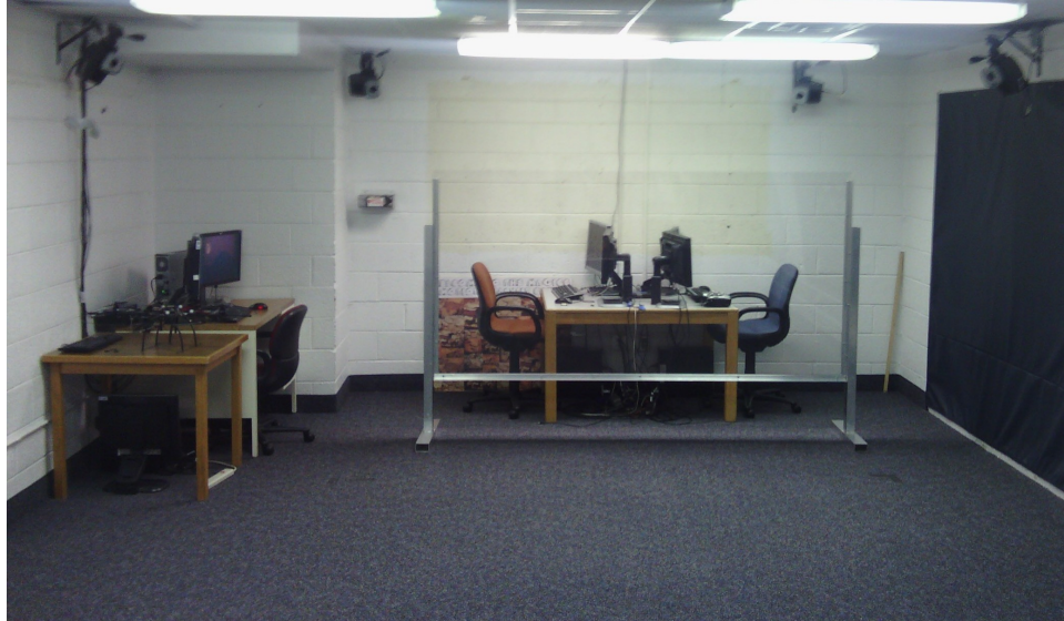
Figure 3. Motion Capture Environment. Here is the motion capture environment where all the testing was conducted for this research. We use a motion capture system from Motion Analysis. The system provides 6DoF pose information at 200 Hz with sub-degree and sub-millimeter accuracy.
