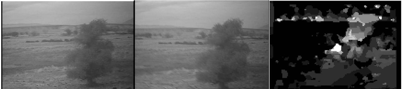
**Figure 4:** Two frames (left, middle) from a sequence of images taken directly from a camera onboard a UAV while it is flying towards a tree. The recovered depth is shown (right).
