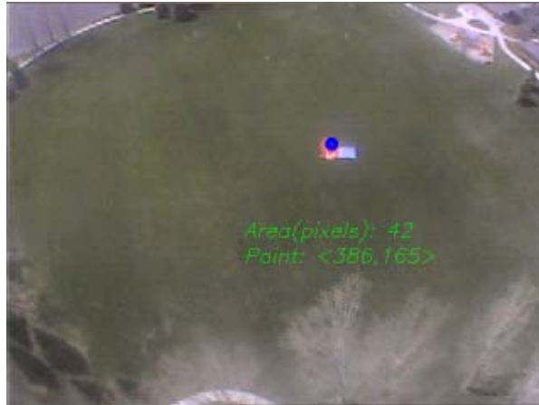
Figure 11: The ground station processes video by color segmentation to find the location of the red cloth.
