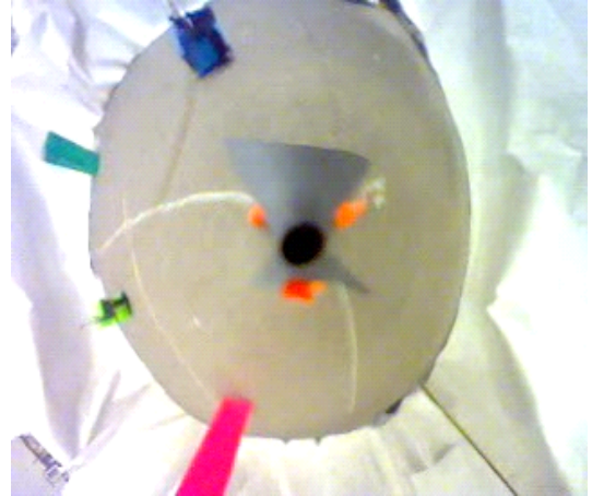
Fig. 13 This figure shows the omnidirectional camera snap shot taken from the orange robot. The snap shot shows the 360° view of the experimental area. It can be seen that other two robots and two landmarks are clearly visible in the image plane. The bearing from the robots and landmarks in the image plane can be computed using color segmentation.
