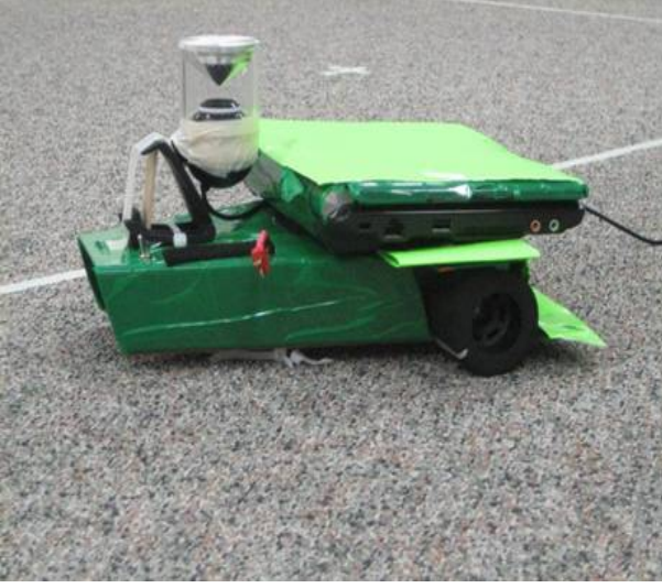
Fig. 11 The Stinger robot. This robot is equipped with a serialize controller, two wheel encoders, an omnidirectional camera, and Asus EEE computer.
