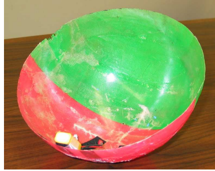
Figure 16 Hemispherical drogue used in preliminary flight tests
