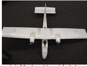
(a) Mothership with 1.4 m wing span, twin props and cable release mechanism.
