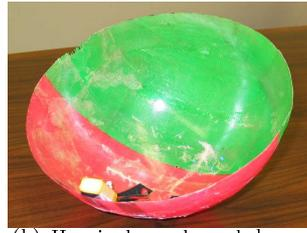
(b) Hemisphere-shaped drogue with 30 cm diameter made of reinforced plastic.
