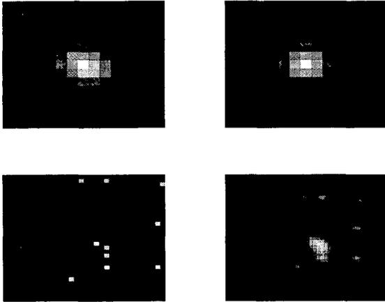
Figure 1. Image to be restored. Top left: Actual blur psf formed as an elliptical Lorentzian function on a GGMRF residual halo producing a realistic AO low-pass “mottled” halo field. Top right: Circularly symmetric Lorentzian blur model to be used as the reference mean,  $\mu_h$ . Bottom left: Actual truth image. Bottom right: Observed blurred, noisy output data.
