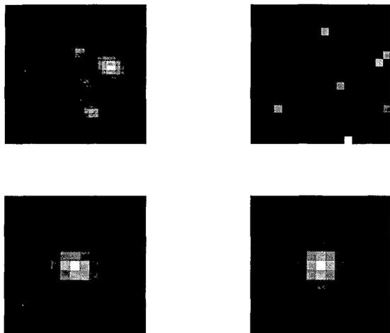
Figure 3. Second example. Top left: Observed blurred, noisy output data. Top right: Actual truth image. Bottom left: Actual blur psf. Bottom right: Circularly symmetric Lorentzian reference mean.
