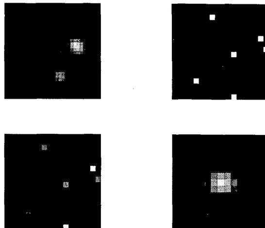
Figure 4. Second example, first restoration. Top left: Restored image blurred with restored blur psf. Top right: Restored activity matrix. Bottom left: Restored input image. Bottom right: Restored blur psf.
