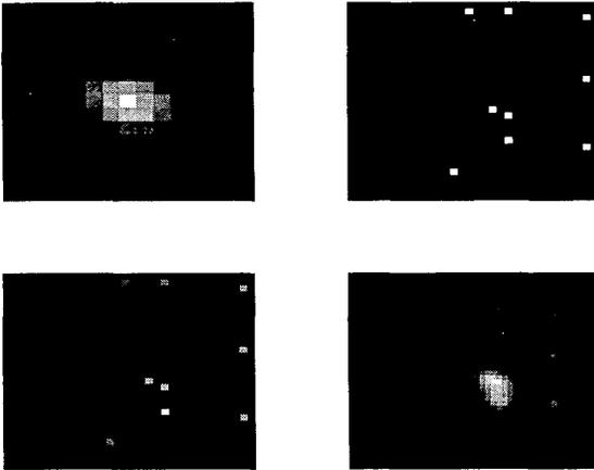
Figure 2. Restoration results. Top left: Estimated blur. Top right: Restored activity matrix. Bottom left: Restored input image. Bottom right: Restored image blurred with restored blur psf. Compare with Figure 1.
