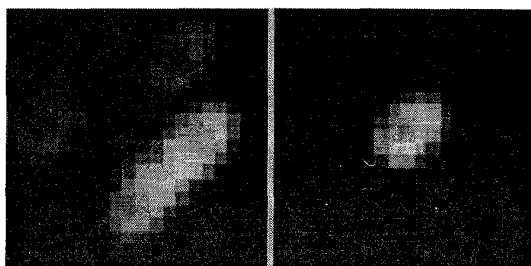
Figure 3. Star cluster image from the CWRU/NOAO observatory, with 2.1 arcseconds resolution per pixel. a) [left] blurred image. b) [right] psf estimate from an isolated star in the same frame.
