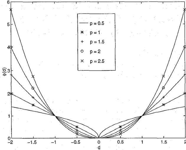
Fig. 1. Potential function of GGMRF for different values of  $p$ . Note that  $x = d_{s,t}$  in this figure.
