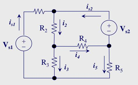
**Example2**: using KCL find  $i_{s1}$  and  $i_{s2}$
