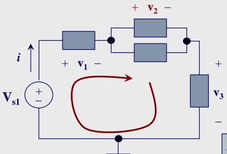
**Source**: loop travels from – **to** + terminals
