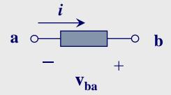
Since *i* is going from + to – energy is being absorbed by the element
