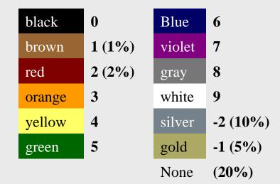
**Example2**: what resistor has a value of 6.2M  $\Omega$ ?
