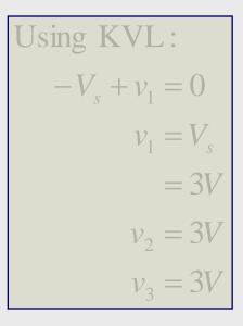
**Example6**: find the voltages and resistances of  $\mathbf{R_1}$ ,  $\mathbf{R_2}$ ,  $\mathbf{R_3}$  $\mathbf{V_s} = 3 \text{V}$ ,  $\mathbf{i_1} = 0.2 \text{mA}$ ,  $\mathbf{i_2} = 0.4 \text{mA}$ ,  $\mathbf{i_3} = 1.2 \text{mA}$
