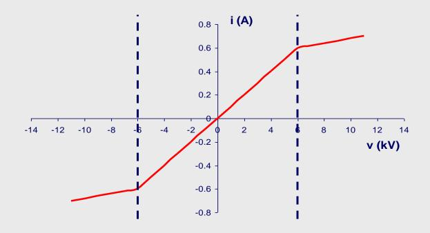
◆ Example3: What is the resistance of the element with the following *i*—v characteristic?
