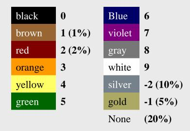
**Example2**: what resistor has a value of 6.2M  $\Omega$ ?
