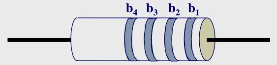
Resistor Value =  $(b_1b_2) \times 10^{b_3}$
