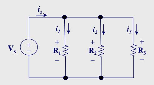
**Example6**: find the voltages and resistances of  $\mathbf{R_1}$ ,  $\mathbf{R_2}$ ,  $\mathbf{R_3}$   $\mathbf{V_s} = 3 \, \text{V}$ ,  $\mathbf{i_1} = 0.2 \, \text{mA}$ ,  $\mathbf{i_2} = 0.4 \, \text{mA}$ ,  $\mathbf{i_3} = 1.2 \, \text{mA}$
