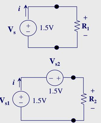
◆ Example4: With a ¼ W rating, what is the minimum resistor size (**R**) that can be used in the following:
