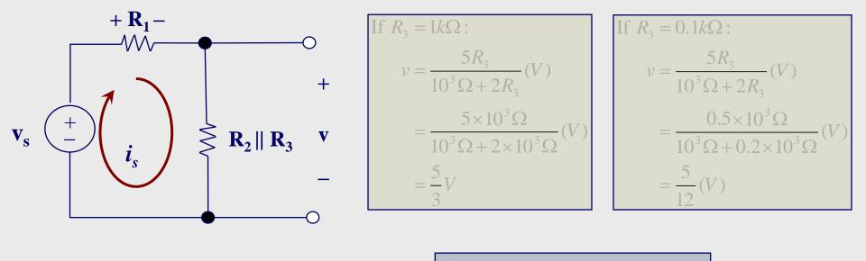
NB: notice how R<sub>3</sub> controls v
