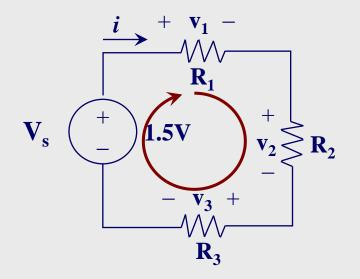
$$\begin{aligned} -V_s + v_1 + v_2 + v_3 &= 0 \\ V_s &= v_1 + v_2 + v_3 \\ &= (i \cdot R_1) + (i \cdot R_2) + (i \cdot R_3) \\ &= i \cdot (R_1 + R_2 + R_3) \\ &= i \cdot R_{EQ} \\ R_{EQ} &= \frac{V_s}{i} \end{aligned}$$
