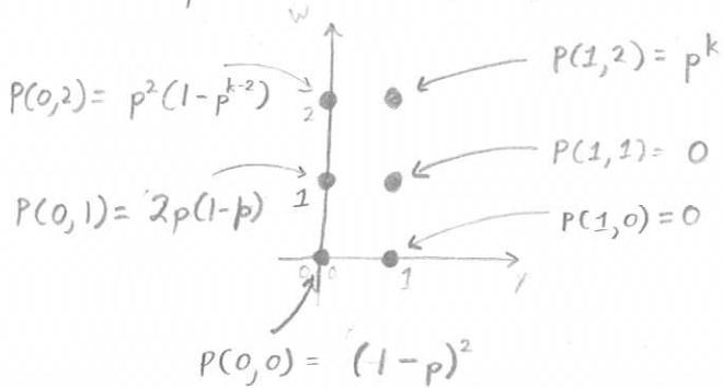
$$\begin{aligned} \sum P(\underline{Y}, \underline{W}) &= \\ &= p^k + p^2(1-p^{k-2}) + 2p(1-p) + (1-p)^2 \\ &= p^{k+2} + p^2 - p^{k+2} + 2p^2 - 2p^{k+1} + 1 - 2p^2 + p^2 \\ &= 1. \end{aligned}$$
