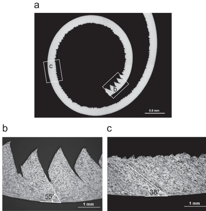
Fig. 9. Cross-sections of chip with mixed segmented and continuous chips at a cutting speed of 16 m/min, depth of cut of 1.50 mm and feed of 0.280 mm.
