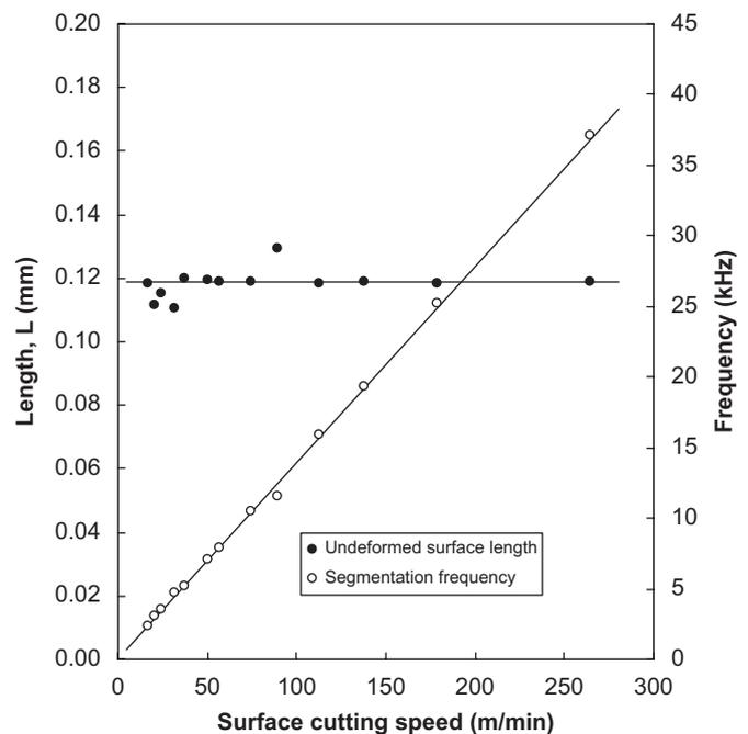
Fig. 10. Effect of cutting speed on undeformed surface length and segmentation frequency.
