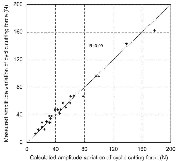
Fig. 12. Correlation between the measured and calculated variation in amplitude of cyclic force due to chip segmentation.
