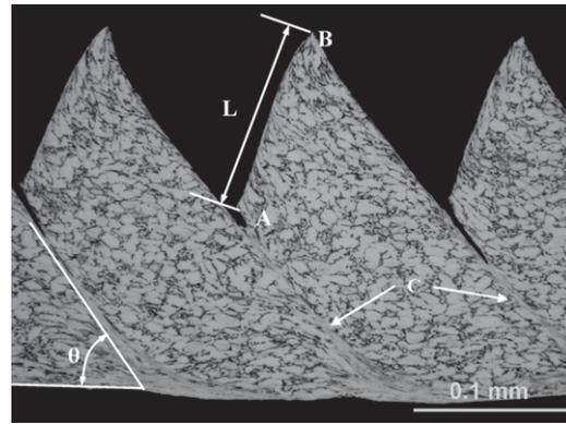
**Fig. 2.** Cross-section of a typical segmented chip in machining of Ti6Al4V alloy.
