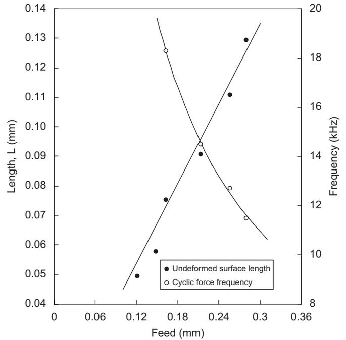
Fig. 5. Effect of feed on the chip morphology and cyclic force frequency at a cutting speed of 75 m/min.
