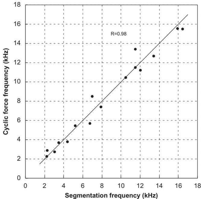
Fig. 11. Correlation between the cyclic force frequency and chip segmentation frequency for different cutting speeds and feed rates.
