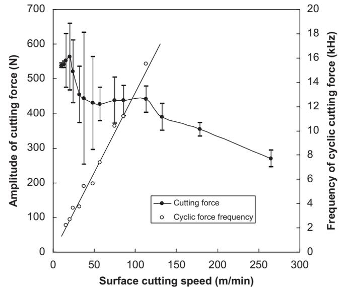
Fig. 6. Effect of cutting speed on the amplitude of force and force variation and variation of frequency at a feed of 0.280 mm and depth of cut of 1.50 mm.
