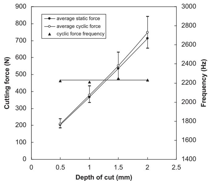
Fig. 8. Variation of static and dynamic cutting force and cyclic force frequency with depth of cut at a cutting speed of 16 m/min and feed of 0.280 mm.
