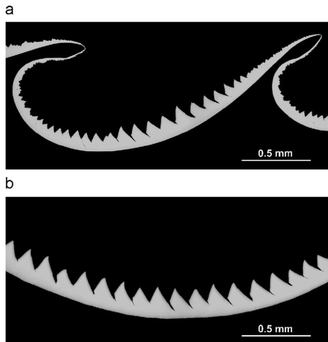
Fig. 4. Chips made at a feed rate of (a) 0.054 mm and (b) 0.280 mm and a cutting speed of 75 m/min.
