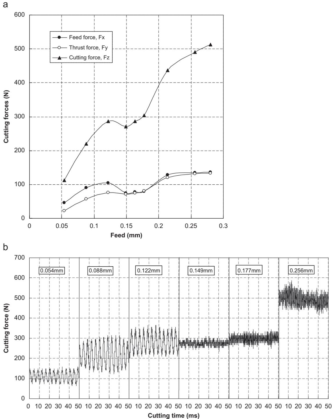
Fig. 3. Effect of feed on the (a) cutting forces and (b) amplitude variation of cutting force at a cutting speed of 75 m/min.
