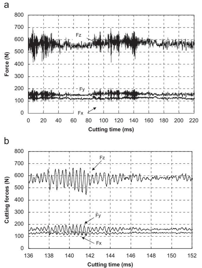
Fig. 7. (a) Variation in cutting forces with time at cutting speed of 16 m/min, depth of cut of 1.50 mm and feed of 0.280 mm, (b) is extracted from (a) to show more details.
