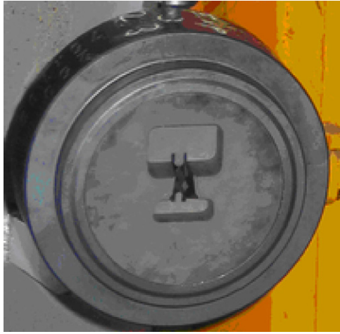
Fig. 3 – Example of a double-pocket die used in extrusion experiments.
