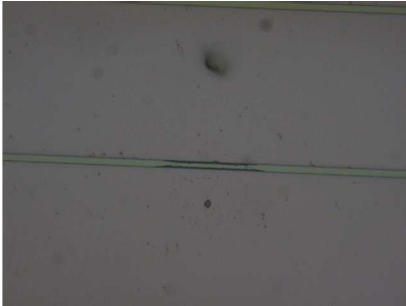
Figure 6.9: Defect on the 8th waveguide of the 1 \times 8 105^\circ TBSN
