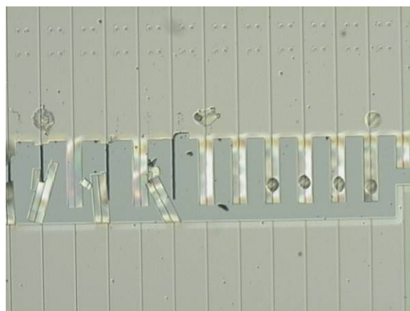
Figure 2-24: Broken MCLs during a test run with the GIX Microplotter II.
