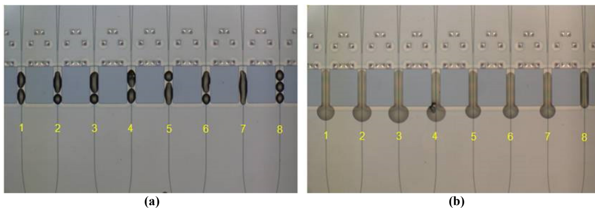
Figure 3-6: 8-PMCL array spotted with various BSA solutions (a) before and (b) after 19 hours of incubation at room temp with the first 7 hours ramping from 24 to 94 %RH.
