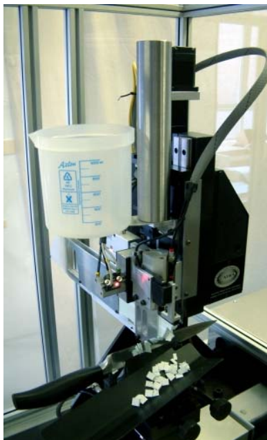
Figure 1: The CATRA Edge Retention Tester, along with a sample data plot from ERT Testing (from [7]).
