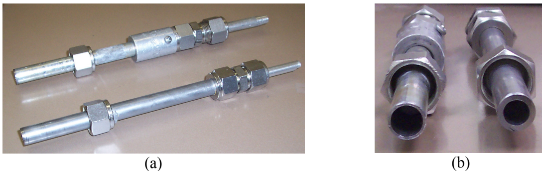
Figure 4.5. Two views of the feeder tube assemblies of different internal diameter.
