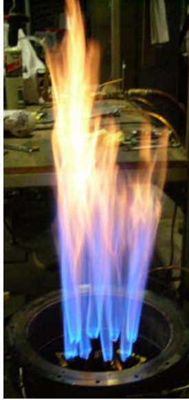
Figure 2-5: Modified flame holders in operation (cone removed)
