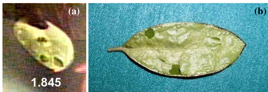
Figure 5.7. (a) Bursting manzanita during reaction in FFB. Video in Appendix D. (b) Upper surface of burst manzanita leaf. Sample was removed from FFB after bursting occurred. Number indicates the time difference (s) from the initial time of the experimental run.
