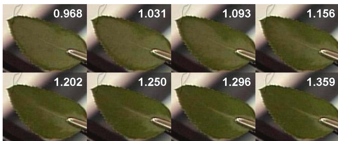
Figure 5.3. Color change sequence for a manzanita leaf. Numbers indicate the time difference (s) from the initial time of the experimental run. Video in Appendix D.
