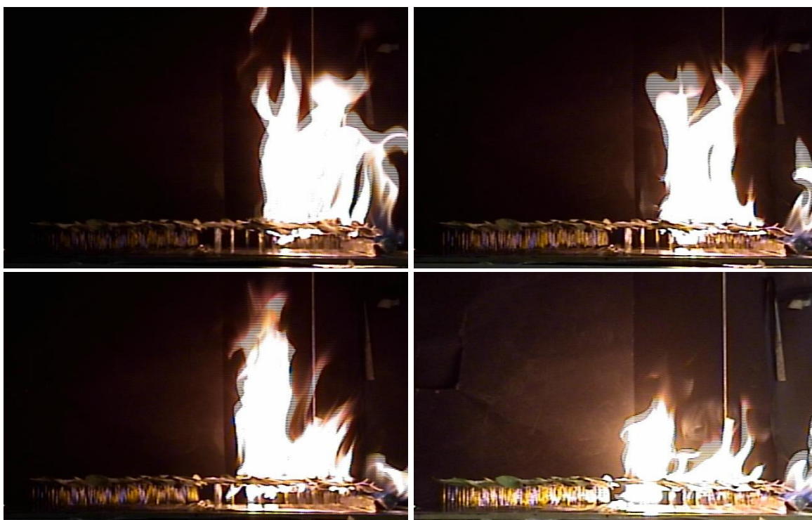
Figure E-9. Skewered leaf Experiment 2 showing flame extension below the leaf surface before fire crosses the 1.5 cm gap.
