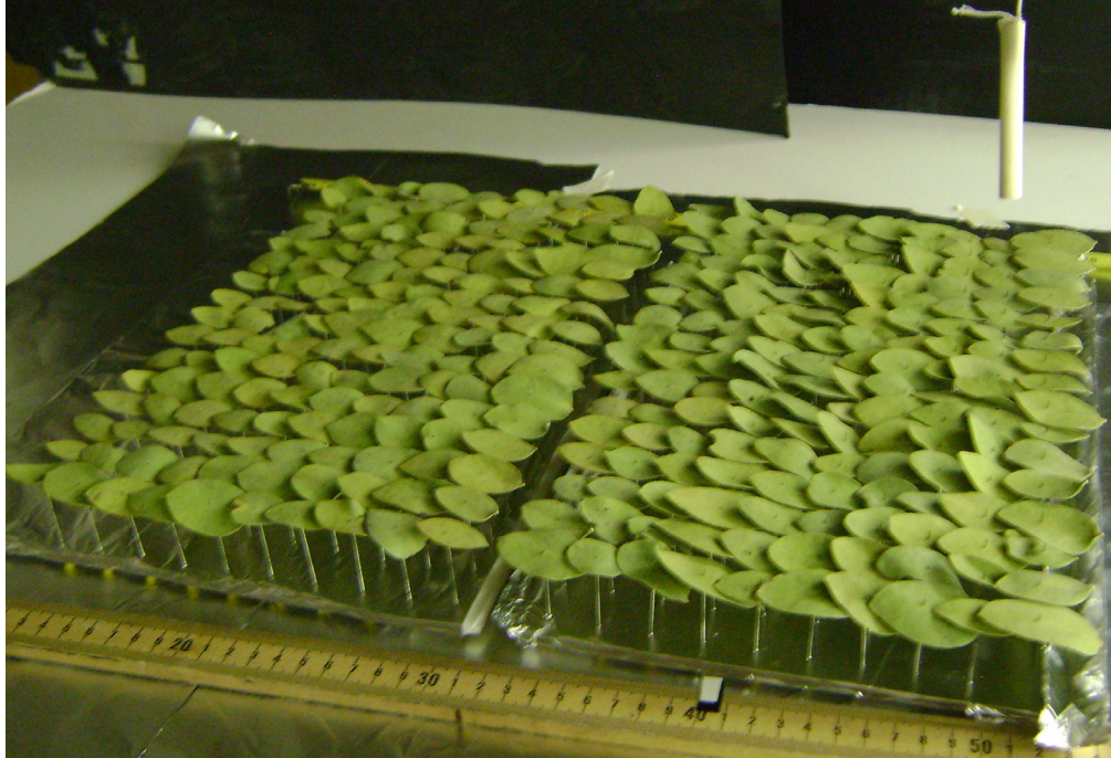
Figure E-6. Skewered leaf Experiment 2 with a 1.5 cm gap prior to ignition.
