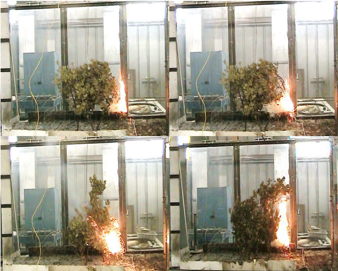
Figure 4-4. Shrubs just after excelsior ignition but before starting the fan for Riverside 2009 manzanita Runs 1 (top left), 2 (top right), 3 (bottom left), and 4 (bottom right). The striped stick at the left of each image marks 25 cm intervals. Viewed through open doors from the same perspective as Figure 4-9.
