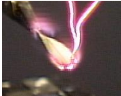
Figure 33. Photos of ignition of Big Sagebrush. These samples had a moisture content of 113%.
