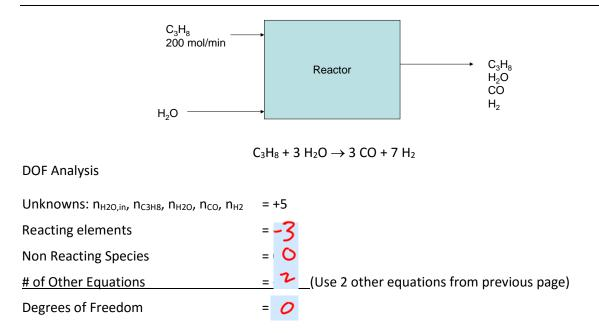
From fractional conversion and % Excess H2O, n<sub>C3H8</sub> = 70 mol/min, n<sub>H2O,in</sub> = 750 mol/min
