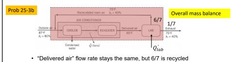
$$\dot{m}_{in,recycle} = \frac{1}{7} \dot{m}_{in,norecycle}$$
