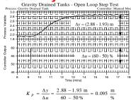
Steady state process gain has a: size (0.095), sign (+0.095), and units (m/%)
