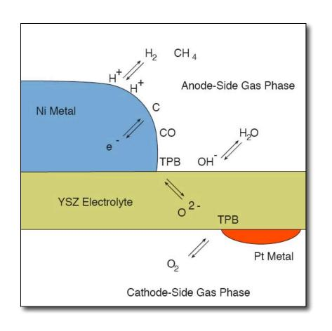
Phases and interfaces involved in a hypothetical solid-oxide fuel cell simulation
