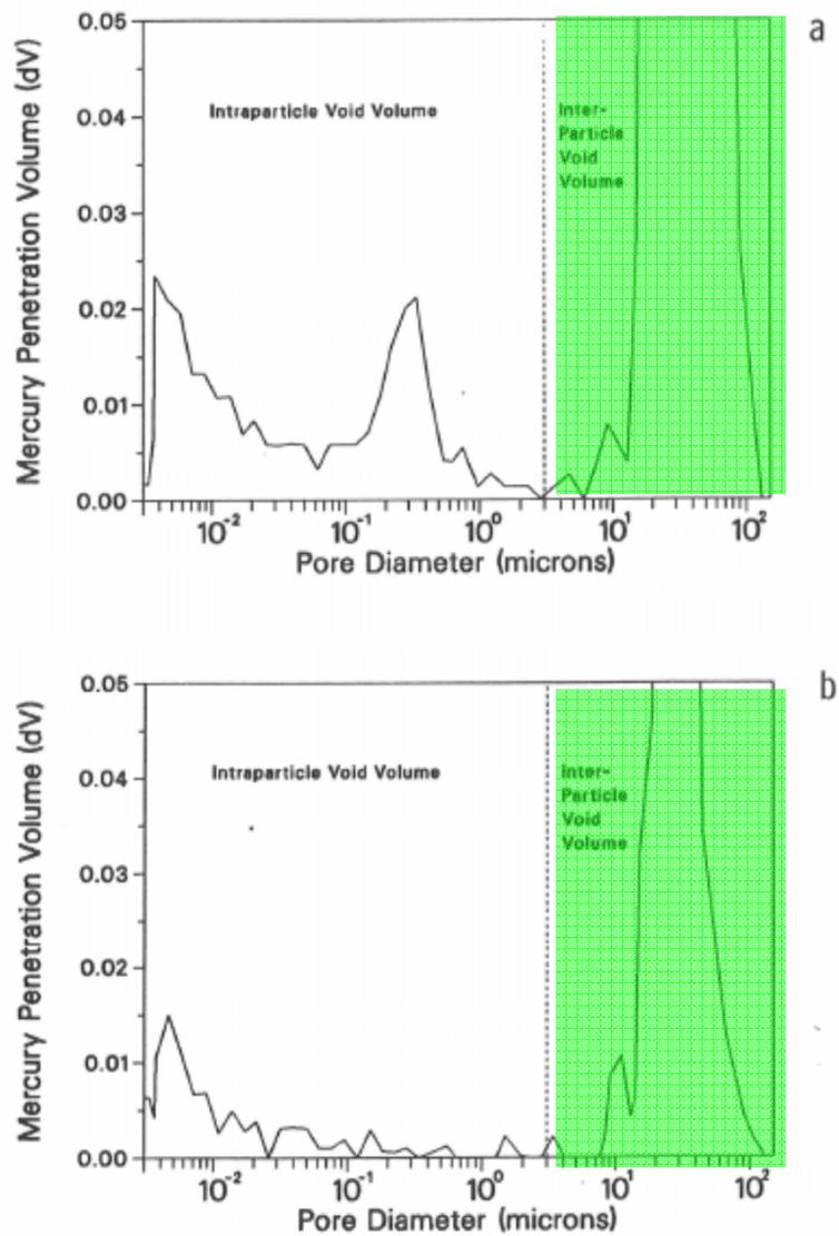
Figure 2. Incremental penetration volume from mercury porosimetry analysis of (a) Sphero carb particles (125 - 149  $\mu\text{m}$ ), and (b) PSOC 1415d Pittsburgh #8 high volatile bituminous coal particles (106-125  $\mu\text{m}$  size fraction).
