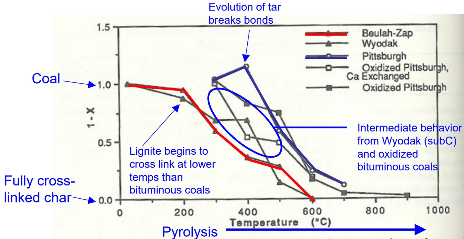
**Figure 50.** Comparison of solvent-swelling ratios for some Argonne premium coals at a series of pyrolysis final temperatures. Effects of oxidation and minerals on cross-linking behavior are shown for the Pittsburgh coal. The Beulah-Zap and Wyodak coals were pyrolyzed with a heating rate of 30 K/min while the Pittsburgh coal sample were pyrolyzed with a heating rate of 0.5 K/s (Solomon *et al.*, 1990).
