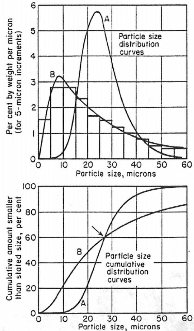
FIG. 8-1. Particle-size distribution curves for simple powders.
