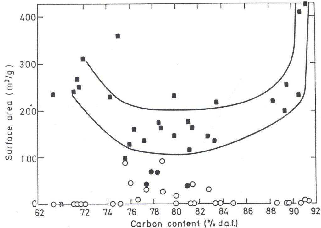
Figure 1 Variation of nitrogen and carbon dioxide surface areas of coals with carbon content
