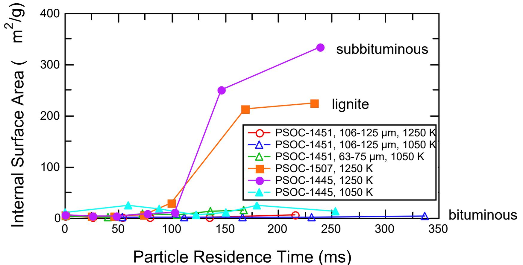
Internal surface areas of char particles from different coals as a function of residence time, as measured by the N<sub>2</sub> BET method.
