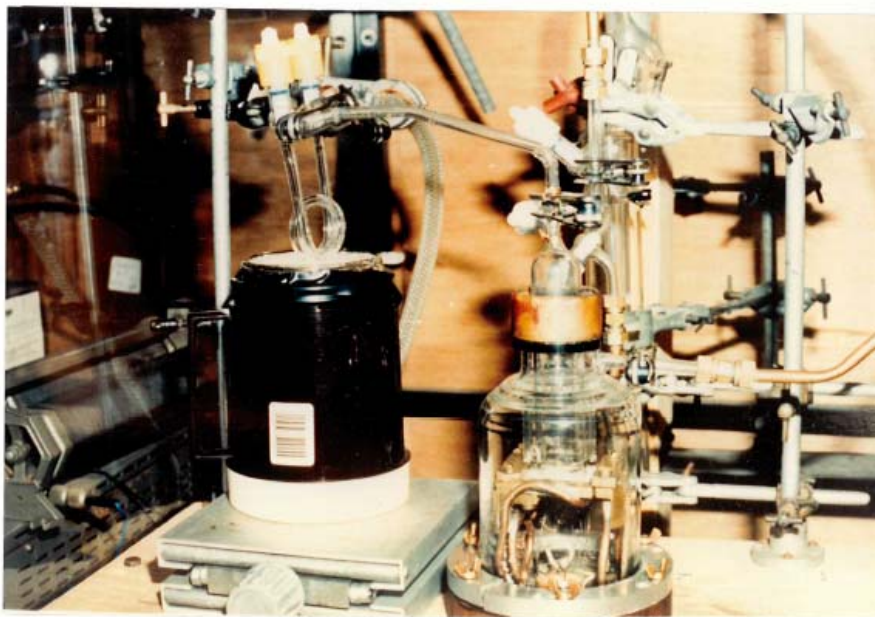
Fig. 3.3 The last development prototype reactor, assembled with the sealable trap in position. (Photo. L. Moulder)
