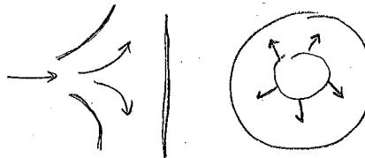
$$Q = 2\pi r_1 b_1 v_{1,n} = 2\pi r_2 b_2 v_{2,n} \quad (\text{radial velocity is carrying fluid out of turbine})$$
