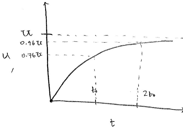
So, when  $t = 2t_0$ ,  $u$  is 96% of the way to being  $\alpha$ . This means  $\alpha$  is the terminal velocity.  $t_0$  should give us our intuition. Let's look at it again.
