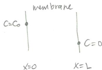
$$\begin{aligned} * \frac{\partial c}{\partial t} &= D \frac{\partial^2 c}{\partial x^2} & c(0,t) &= c_0 \\ & & c(L,t) &= 0 \\ & & c(x,0) &= 0 \end{aligned}$$
