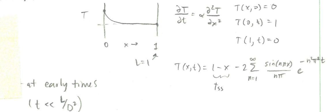
$$\frac{\partial T}{\partial t} = \alpha \frac{\partial^2 T}{\partial x^2} \quad T(x, 0) = 0$$
