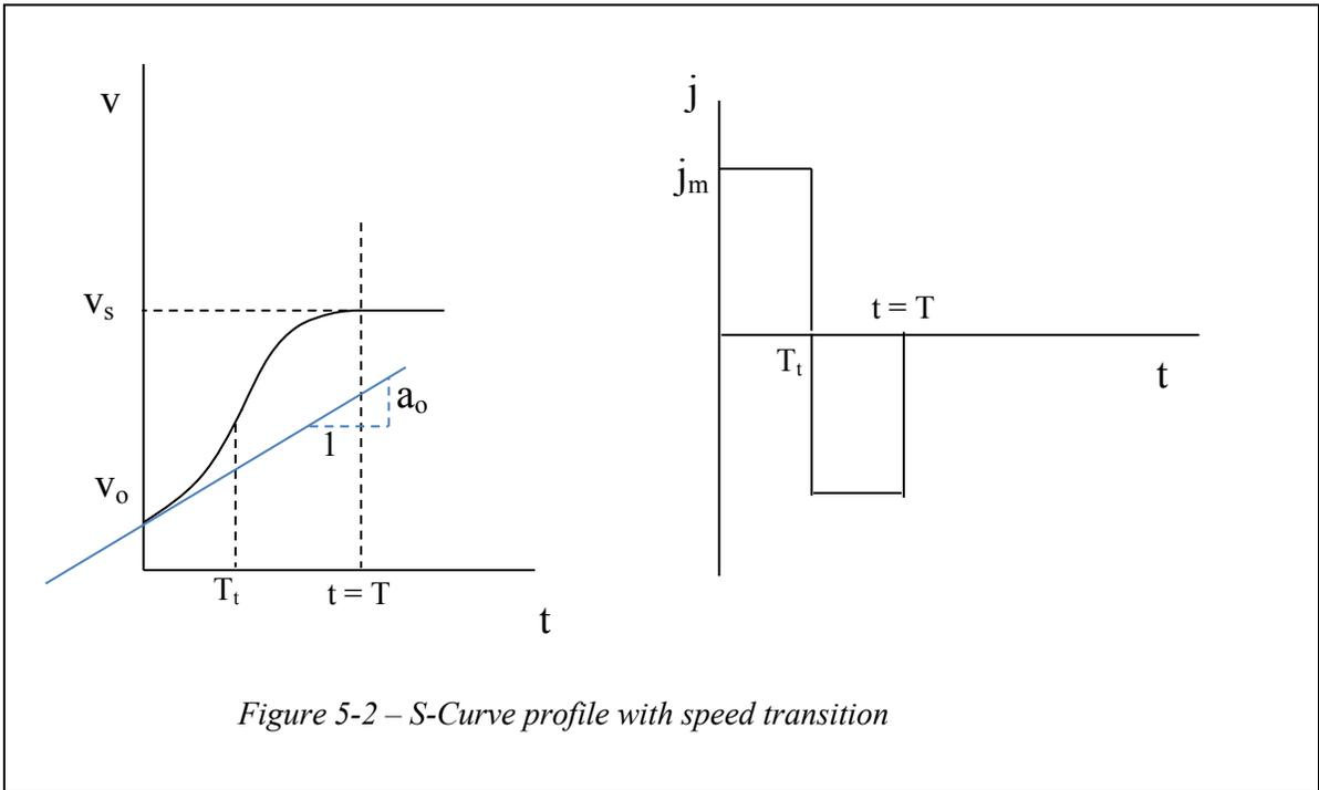
Figure 5-2 – S-Curve profile with speed transition
