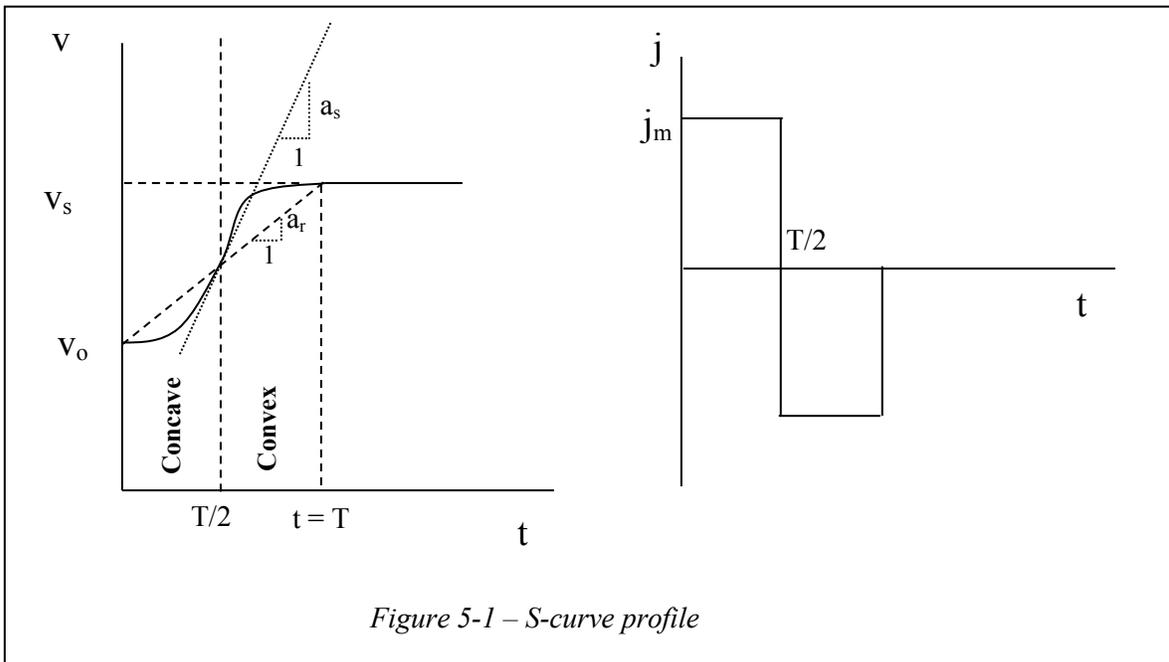
2. The maximum S-curve accel (midpoint of accel period and specified as  $a_s$ ) exceeds the constant ramp accel value which is constant and specified as  $a_r$ . Thus, the S-curve accel must be checked against the robot maximum and adjusted accordingly.
