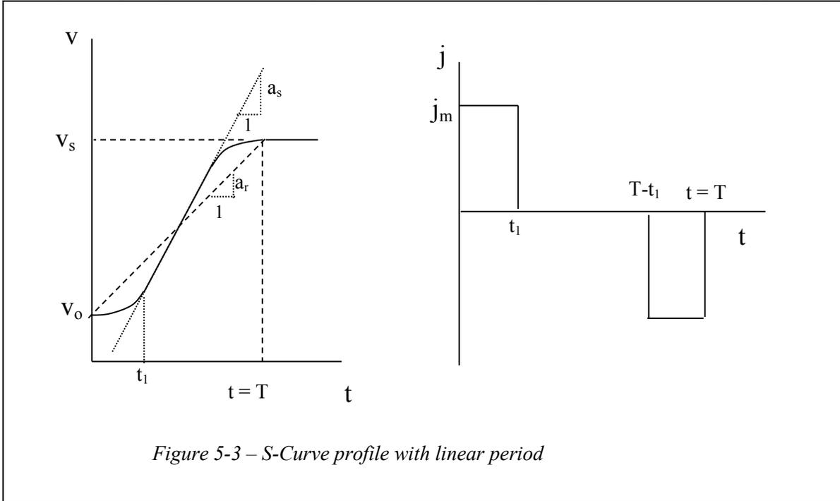
Figure 5-3 – S-Curve profile with linear period
