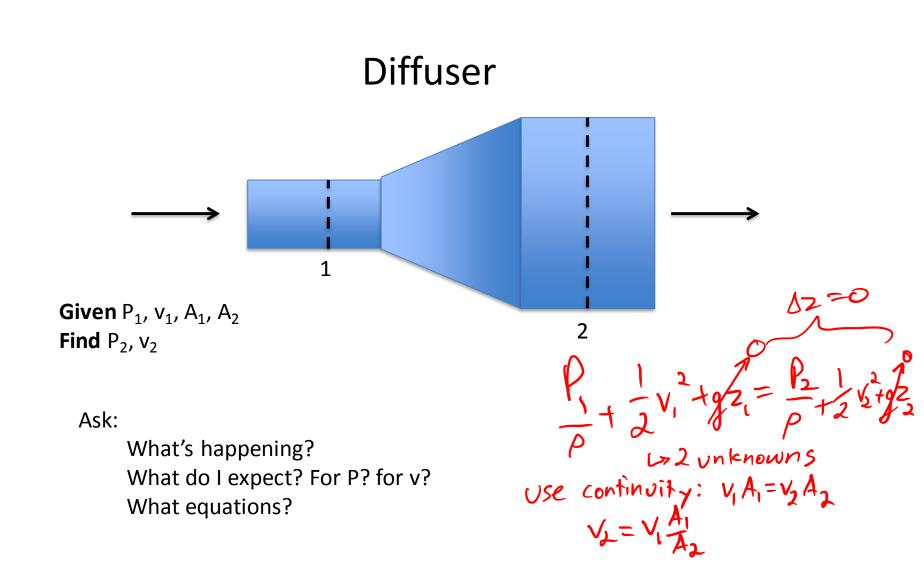
$\frac{1}{p} + \frac{1}{2}v_1^2 = \frac{1}{p} + \frac{1}{2}v_2^2 + \frac{1}{p}(1+\frac{1}{2})^2$  $\frac{P_{2}}{P} = \frac{P_{1}}{P} + \frac{V_{1}v^{2}}{V_{1}} - \frac{V_{2}v^{2}}{A_{1}} + \frac{A_{1}^{2}}{A_{2}}$  $P_{2} = P_{1} + \frac{1}{2} p v_{1}^{2} - \frac{1}{2} p v_{1}^{2} \frac{A_{1}^{2}}{A_{2}^{2}}$
