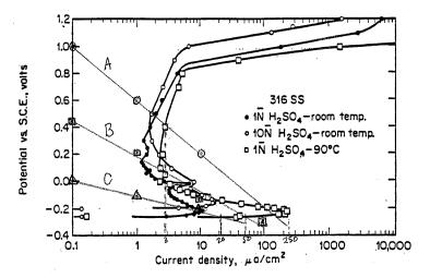
(e) Suppose your solid baffle is made of 316 SS, with dimensions 5 x 5 x 0.2 cm. If it were placed in solution A at 90°C, how long would it take to completely corrode the baffle away? (Assume that the specific gravity of 316 SS is 8.02.)
