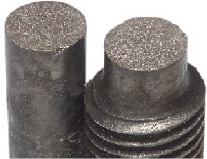
brittle fracture - totally brittle - flat surfaces
