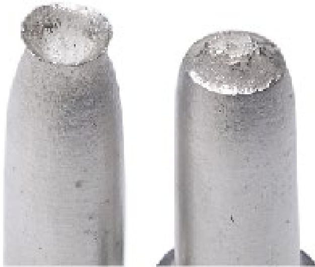
cup-and-cone fracture - moderately ductile
