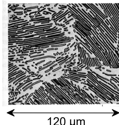
Result: Pearlite = alternating layers of  $\alpha$  and  $Fe_3C$  phases
