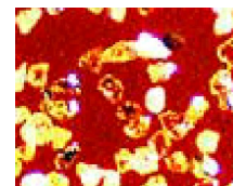
polycrystalline diamonds in a resin matrix.
