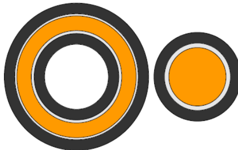
Annular fuel rod cross section (left) vs traditional solid fuel rod (right)
