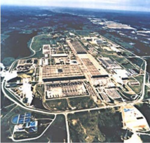
Relies on molecular effusion (the flow of gas through small holes) to separate U-235 from U-238. The lighter gas travels faster than the heavier gas. The difference in velocity is small (about 0.4%). So, it takes many cascade stages to achieve even LEU.
