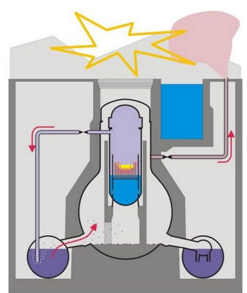
Unit 1 reactor building; top portion damaged from earlier explosion
