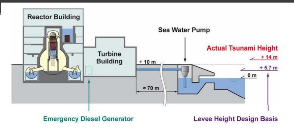
At Fukushima Daiichi, countermeasures for tsunamis had been established with a design basis height of 5.7 m above the lowest Osaka Bay water level.
