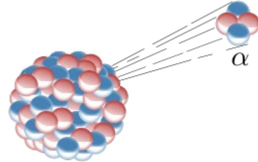
Energies of alpha and daughter particles are fixed, and alpha particle energy is uniquely associated with isotope.
