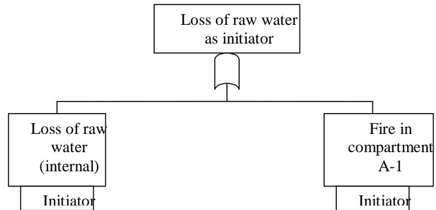
**Example of new logic with a fire-induced loss of raw water initiating event**
