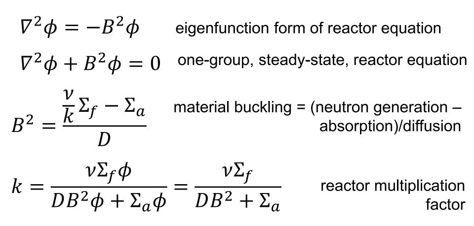
multiplication factor = neutron generation rate/(leakage + absorption)
