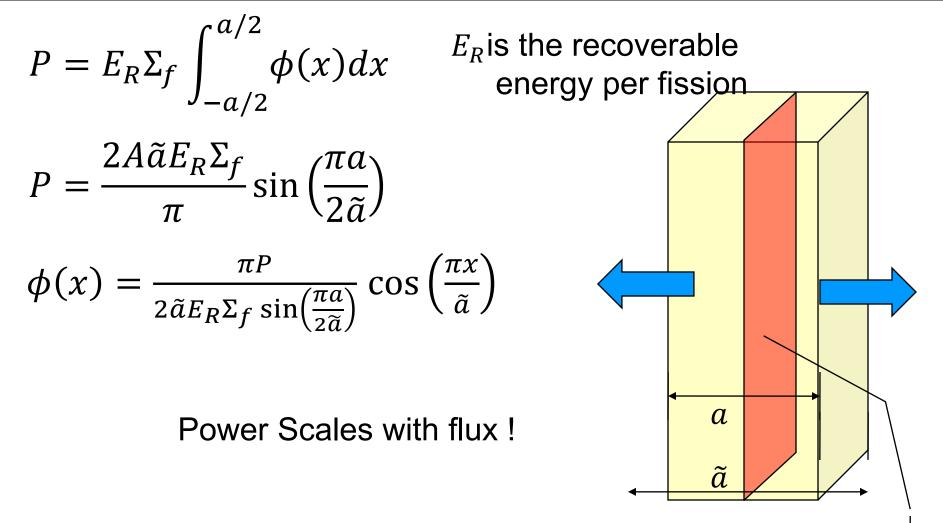
Infinite plane indicates no net flux from sides
