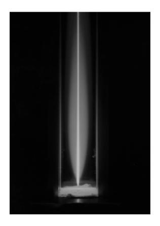
Figure 3.2. A photograph of the visible soot cloud.
